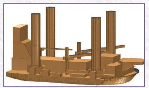
Watertight subdivision of hull is an art to meet Damage and Residual Stability requirements, while accommodating preferred layouts and segregation of spaces desired from Owners. We are specialised to ensure best watertight subdivision with minimum watertight compartments.
